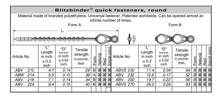
The Allplastik-Blitzbinder® quick fasteners made of premium quality polyethylene have a special closure which, when combined with a round profile, guarantees maximum strength and reliable closing and can also be opened again at any time. In addition to its function as a fastener, the dual closure design of the Allplastik-Blitzbinder® quick fasteners allow a hanging loop to be formed.
